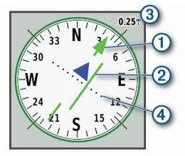
The course pointer 1 indicates your relationship to the course line leading to the destination. The course deviation indicator (CDI) 2 provides the indication of drift (right or left) from the course. The scale 3 refers to the distance between dots 4 on the course deviation indicator, which tell you how far off course you are.
