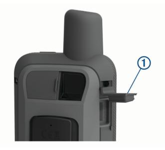
2 Insert the memory card with the gold contacts facing the device screen.
